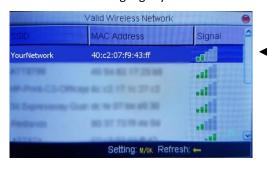
Signal must be at least 2 bars in order to connect properly.
